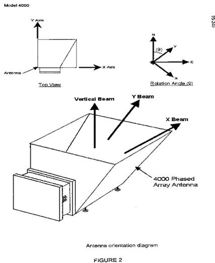
The main reflecting surface is tilted at a 45 degree angle from the vertical, and is sized to allow all three monostatic beams to be transmitted with minimal interference. An **optional area heater**, which covers the surface of the reflector panel, is available for regions with significant snowfall during winter months. The other three sides to the antenna assembly are covered with acoustic absorbing foam to
