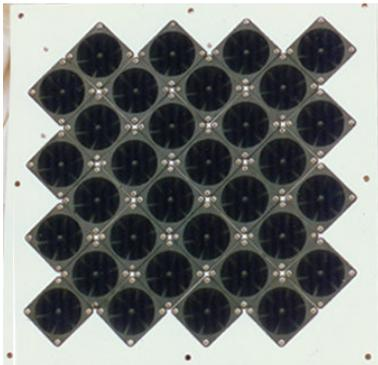
A back-scattered signal is produced by the interaction of the transmitted acoustic steered pulse with small scale atmospheric turbulence. This signal is received by the speaker array. It is analyzed both for energy and frequency content using spectral processing techniques. The energy
