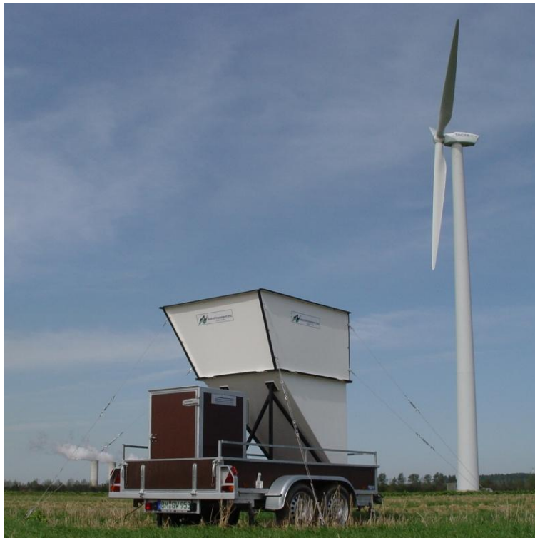
Trailer-based SODAR system during a measurement within a wind farm
