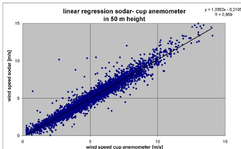
Fig. 2: Linear regression SODAR vs. cup anemometer with offset
