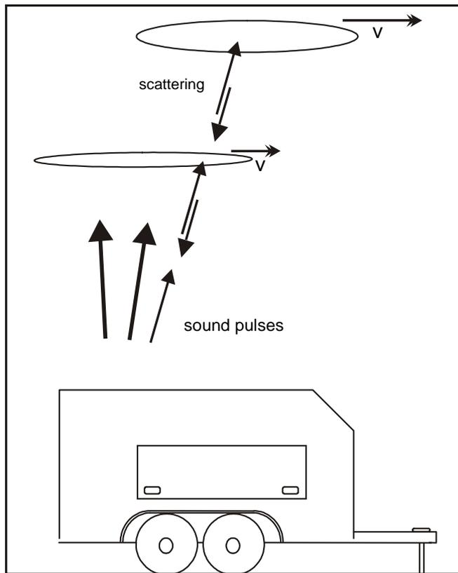
Fig. 1: SODAR operating principle
