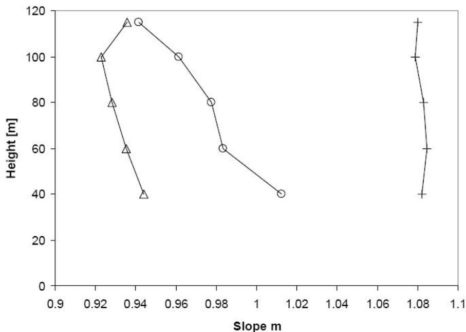
Fig. 6: Height dependence of regression slope vs. mast for 3 different SODARs
