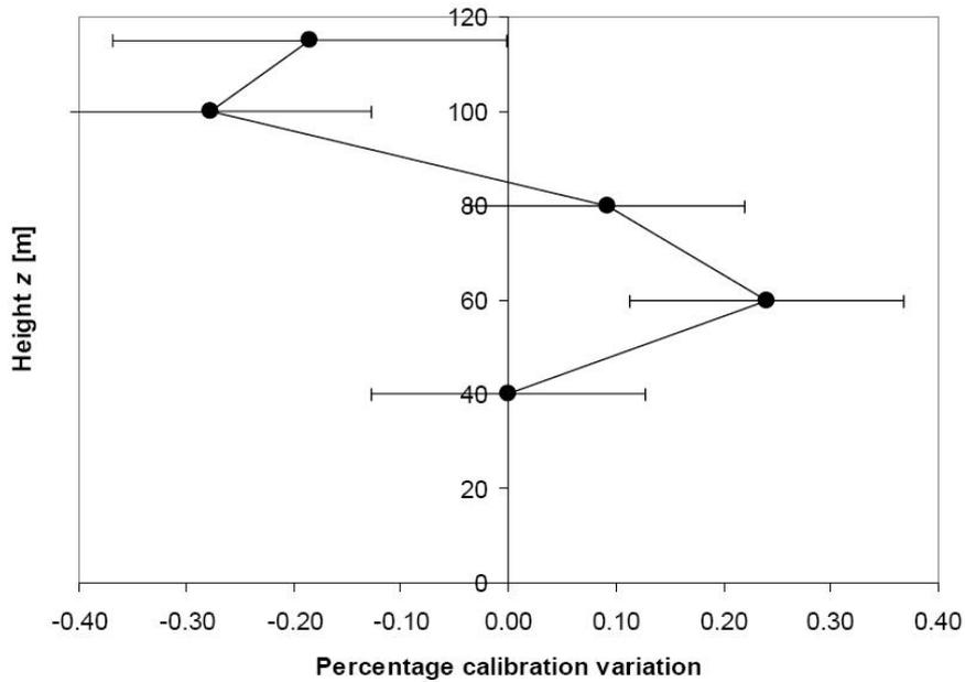
Fig. 7: Height dependence of the variation in calibration for AeroVironment (ASC)
