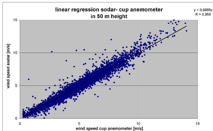
Fig. 3: Linear regression SODAR vs. cup anemometer forced through the origin
